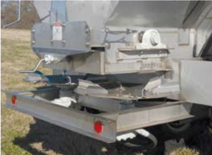
Manufacturing fertilizer spreaders involves intensive use of plasma cutting by Newton Crouch, Inc. A switch to a different consumable saved 50 percent in parts and 20 percent in clean-up.
